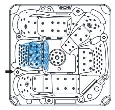
Jet pump 3-nozzle system 2 Located at left seat
