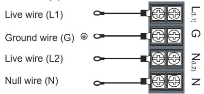
Note: connect the power line according to the above mentioned figure
