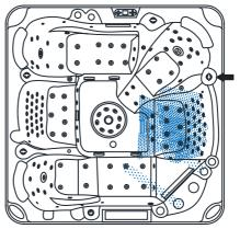
Jet pump 1-nozzle system 1 Located at the right seat
