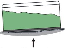
The spa could loss its leveling state because of the sinking of the stones or bricks
