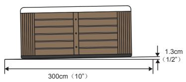
For correct water drainage, the inclination should be 1.3 cm (1/2 inch) / 305 cm (10 inches)
