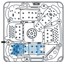
Jet pump 3-nozzle system 1 Located at lower left lying place
