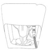
Confirm the inlet valve and reducing valve is open
