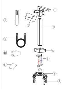
In order to guarantee the water flowing smoothly, pls clean out the mud and sands in the pipe before connecting the inlet pipes.
